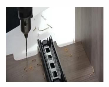
Drill the hole on inside of carcase for connecting L connector
