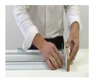
Fix the L connector on profile back side grooving.
