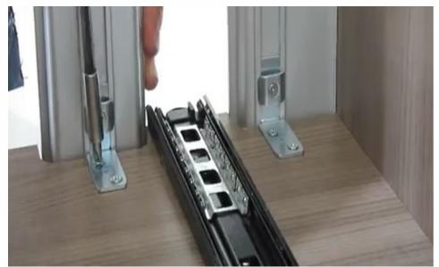
Screw -C connector on the carcase
